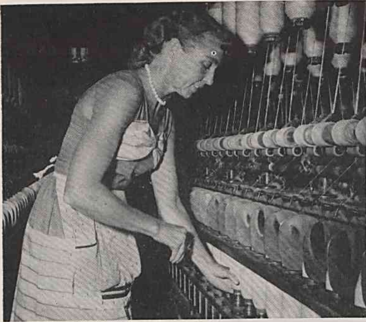
Mabel Akers, Towel Mill spinner, demonstrates how bobbin is grasped firmly to stop spindle and avoid burning hand.
