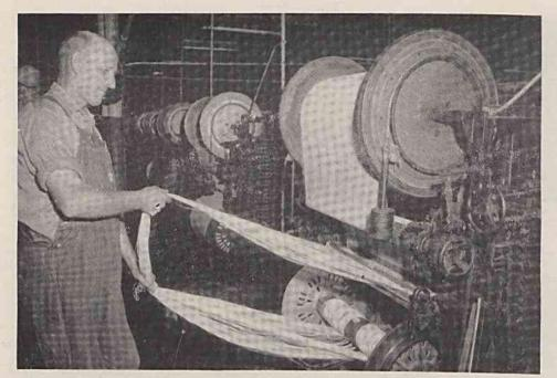
WASTE CONTROL—Charlie Cannaday, lease man at Towel Mill, prepares for warp change. Note that only a minimum amount of yarn remains on the beam. When warps are properly run out, the last good yarn on the beam can be woven into cloth; when warp is cut off too soon this yarn becomes waste.
