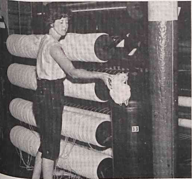
Doreen Minter, card tender, puts roving waste in can where it will be kept separate from waste from other cards and will be fed back into the card before end of the shift.
