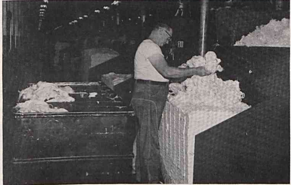
When the waste is collected from all the cards once each shift, it is kept separated in a box truck which has a compartment for each card. Here, Percy Robertson gives close attention as he places waste on pile of stock at hopper.
