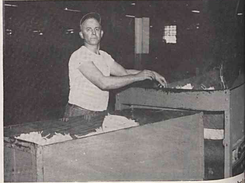
Brody Radford is shown as he examines roving waste which is belatedly processed through a picker prior to being placed back into carding operation.
