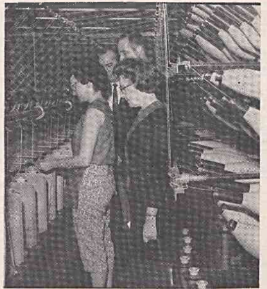
Professor Harrison and students watch Mavis Campbell repair end break on twister.
