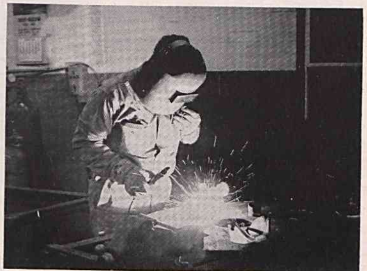
Bobby Shelton practices arc welding. Eyes are protected, helmet and gloves used to avoid burns from ultraviolet rays.
