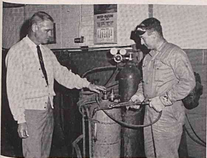
Dwight Wilkinson, foreman, shows Bobby Shelton how to set controls on acetylene and oxygen tanks for safer cutting.
