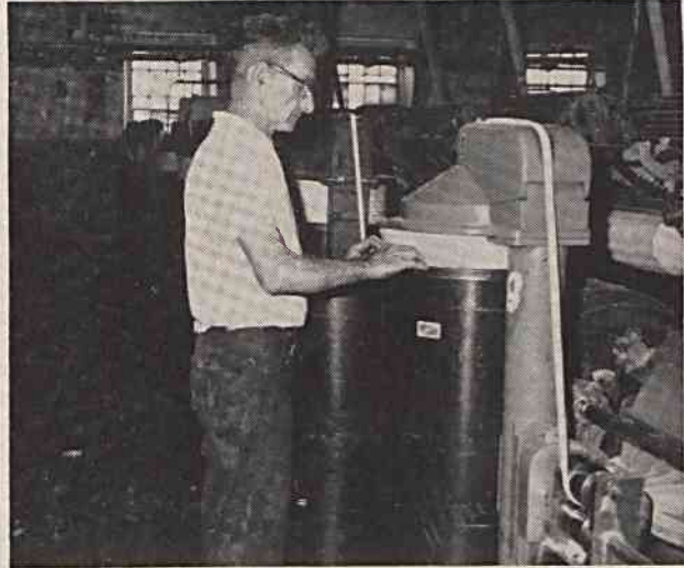
The cards in Worthville mill are equipped with all-metallic wire clothing. Operator here is C. C. Marsh.
