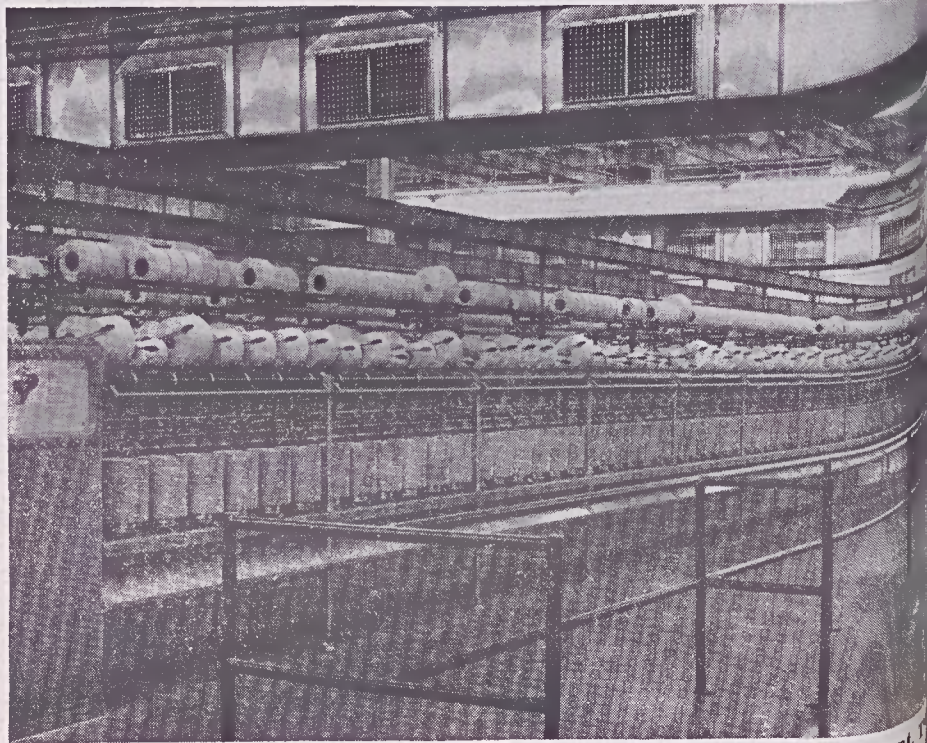
A number of Hamel 2-for-1 twisters were installed as additional equipment. They double, twist and wind the yarn in one operation, delivering package ready.
