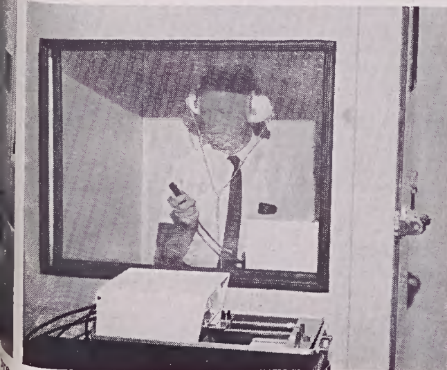
Audiometer, a device for testing hearing, is used in pre-employment examinations and health maintenance.
