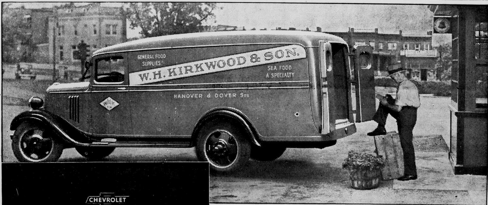
Illustrated: 1 1/2-Ton Panel Truck (131" Wheelbase)
