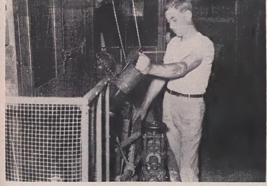
Justice Boyd (Machine Shop) inspects a newly installed guard to protect fingers from the nip rools used in connection with the "Kleersheen" stencil. This guard was designed to prevent the recurrence of a recent accident in which an employee received painfully mashed fingers while attempting to wipe a grease spot from the roll.
