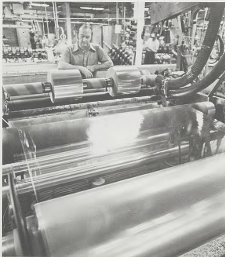
Note the glistening transparency of cellophane. Cellophanes are produced to certain customer specifications because of particular packaging needs. The film is used for baked goods, meats, produce, candies, snack items and others. Cellophane provides an excellent surface for printing. Here, Roy Millwood of the Slitting Section in the Finishing Department is running a set-up of film.
