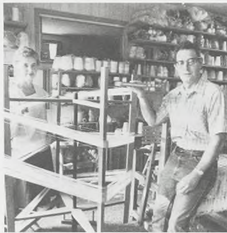
Bob and Barbara Miller demonstrate a warping mill Bob made for his wife's weaving studio, which he also built.
