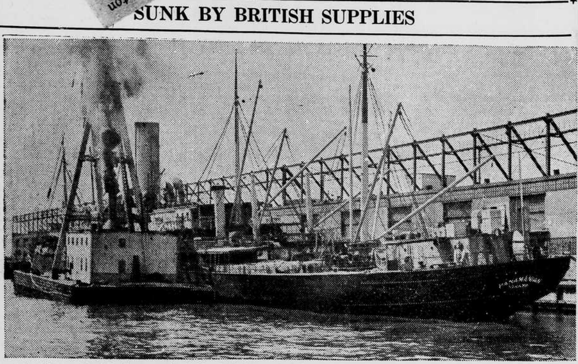
A salvage derrick leans against the 15,575-ton freighter Panamanian after the vessel partially sank recently at a Baltimore pier. The accident, attributed by coast guardsmen to overloading, occurred while loading a general cargo for British ports. The ship is under charter to Arnold Bernstein, refugee German shipping magnate.
