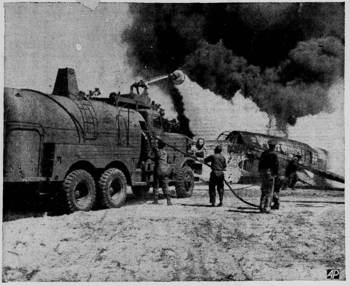
Demonstrating a new method of fighting plane fires, Army firemen operating two huge tank trucks at Jacksonville, Fla., extinguished in two and one-half minutes an obsolete bomber which had been drenched with gasoline and fuel oil and set ablaze. One truck (left) sprays carbon dioxide and the other (not shown) sprays water under tremendous pressure.
