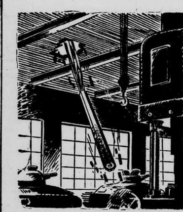
5...THE M-69'S STREAMING TAIL slows its fall to 225 to 250 feet per second—fast enough to pierce the factory roof; slow enough to keep the incendiary bomb from destroying its own mechanism on impact. One of M-69's most effective qualities is its ability to carry fire inside the target...
