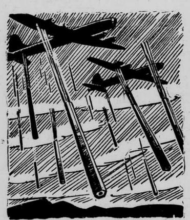
4...DOWN NEAR THE TARGET, each big bomb opens to free its load of M-69's. Each M-69 carries enough of a special jellied gasoline to make a sticky, flaming "pancake" 1/4-inch thick and 3 feet across...ejecting fiery globs which stick to and burn fiercely on any surface they may hit.
