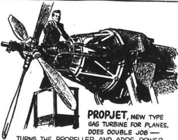
TURNS THE PROPELLER AND ADDS. POWER THROUGH A JET TO THE REAR. EXPERTS SAY PROPJET WILL POWER GIANT TRANSOCEANIC AIR LINERS OF TOMORROW. IT WAS DESIGNED BY GENERAL ELECTRIC ENGINEERS.
