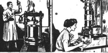
The ultra-centrifuge, which spins at 60,000 revolutions per minute, is a valuable weapon in polio research. When the virus has been precipitated it is studied through the electron microscope, which magnifies 200,000 diameters.
