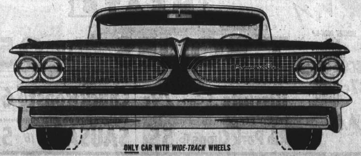
. . . acclaimed by experts as the year's top engineering advance! The wheels are moved out 5 inches for the widest, steadiest stance in America-lower center of gravity for better grip on the road, safer cornering, smoother ride, easier handling. Pontiac gives you roadability no narrow gauge car can offer!
