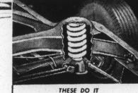
tour big-but-gentle coil springs permit each wheel to "step over bumps as it reaches them. It is this independent action of each wheel that gives Buick its matchless buoyancy on any and all roads.
