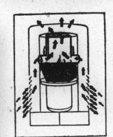
TURNS WASTE INTO WARMTH. Only Heatrola has the famous, patented Intensi-Fire Air Duct. Built right in the path of the flame, it blocks much of the heat ... sends it into the rooms instead of up the flue.
