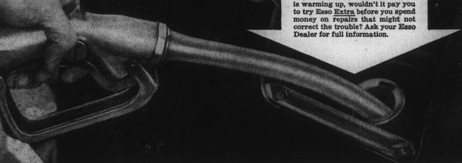
If your car stalls in damp, cool weather (30° to 55°) during the first fifteen minutes of driving, the chances are the cause is carburetor icing. This is not the fault of your car. Mechanical adjustments can't cure it.
