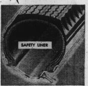
Here is a tire with new principles of design and construction which protects you against dangerous blowouts. In this new safety tire, the tube is replaced by an air-tight butyl Safety Liner that's bonded to the inside of the tire. No tube to pinch, tear or suddenly explode when injury to the tire body occurs. Air loss is so gradual there is ample time for safe, sure stops.
