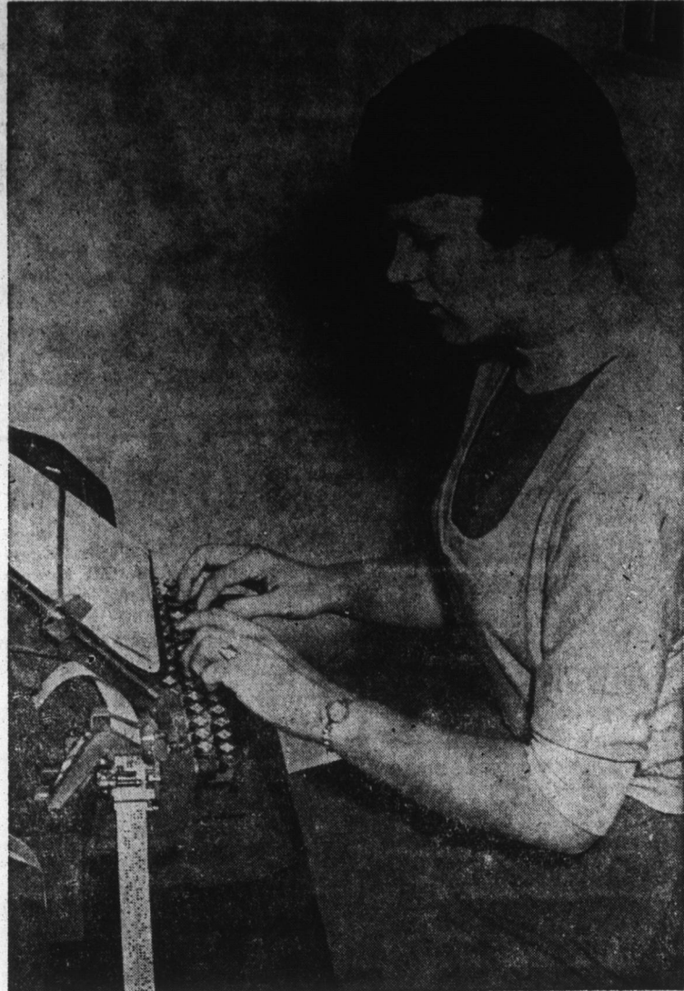
Pretty Jean Sykes of Conway, N. C., is shown operating the keyboard of a teletypesetter perforator, the machine that has opened up an entirely new occupation for women in the newspaper field. The tape from this machine (shown in the lower left hand of the picture) is fed through an apparatus attached to a typesetting machine and automatically sets type for newspapers. Miss Sykes is a student at the Roy Parker School of Printing, Chowan College, Murfreesboro, the only school in the entire South where such training is available. (Chowan College News Bureau photo)
