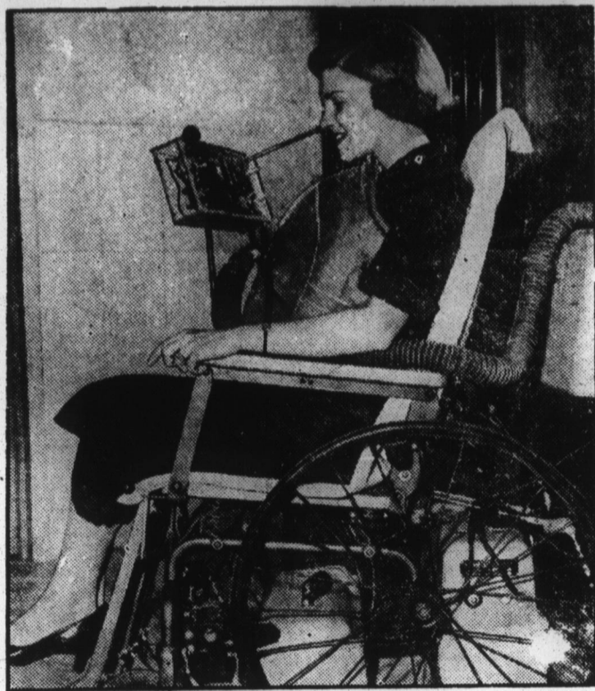
DESIGNED FOR POLIO VICTIMS —Designed for use by nearly paralyzed polio victims who still have control of neck and facial muscles, the motorized chair pictured above is the development of Ed Tilden Atkins, of Chicago, Ill. Instrument panel before the patient's face may be actuated by a stick held in the mouth, protruding rod is nose operated; controls forward-reverse motion of chair. Fashioned of aircraft parts, mechanism is powerful enough to pull portable chest respirator as well as patient, as modeled by Mrs. Barbara Pollard.
