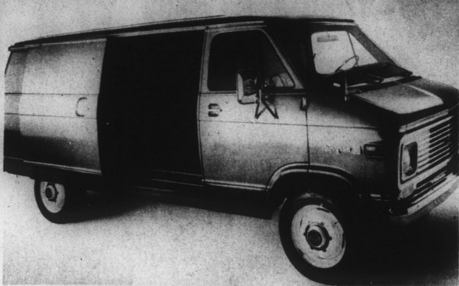
ONE-TON VAN —Featuring a convenient sliding side load door with concealed inside step protected from the weather, the 1971 Chevy-Van is completely redesigned for greater utility and load capacity. Cargo area is greater and a new front extension provides much more convenient engine servicing, as well as more clear floor space and easier access to the load compartment. Wheelbases and bodies are longer, with front wheel location farther forward for easier entry and exit, better ride, and more frontal impact protection for occupants. Chassis improvements include independent front suspension and two-stage leaf rear springs.
