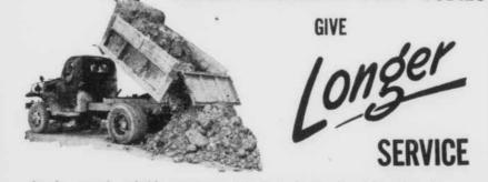
Steady, smooth, reliable operation of Galion's Hydraulic Hoist offers dump truck men maximum efficiency with greater power. Designed for 11/2 ton trucks . . . the Galion Model GH 56 has patented Equalizing Double Arm mechanism to provide low and uniform oil pressure. No strain on truck motor, and three-way valve holds body at any angle. Galion hoists are known to last longer than three or four chassis. It's their immunity to wear and tear that makes them popular with operators.
