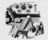
YOU GET CONVENIENCE. The Universal "Jeep" is as easy to drive as a car. Controls are simple and conveniently placed. It has full instrument panel, self starter, conventional pedals and accelerator. You change from 2 to 4wheel drive by merely shifting transfer-case lever. Powerful sealed-beam head-
