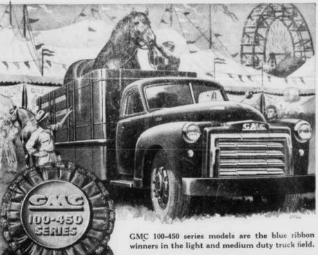
They're Big . . . built to handle gross weights up to 37,000 pounds. They're Strong . . . with wide, deep frames and long, thick, load-supporting springs. They're Better Built . . . with such features as hypoid rear axles, full pressure engine lubrication, Turbo-Top pistons, 3- and 4-speed Syncro-Mesh transmissions, Ball-Bearing Steering.
