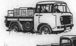
The New Forward Control 'Jeep' FC-150...puts a 74" pickup box on a wheelbase only 81" long.
