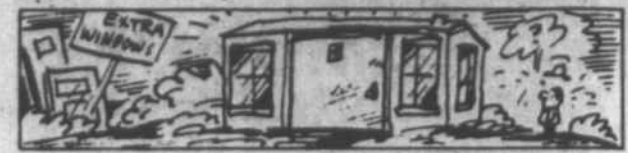
The larger the doors and windows of a home, the greater the chance of heat loss in winter, or heat gain in summer.
