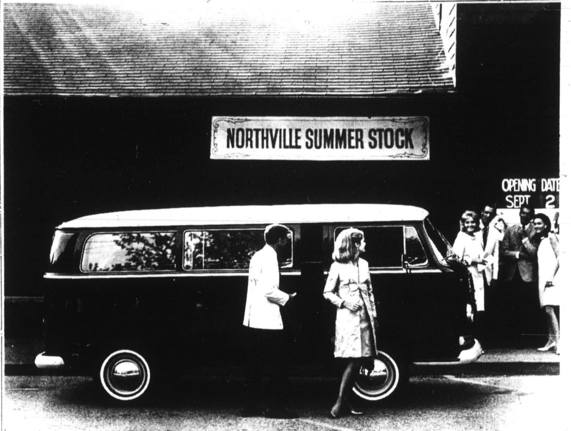
VOLKSWAGEN'S B o x-shaped split-window, and a single, sliding side door eliminates the double hinged doors of earlier models. A sleek exterior appearance is achieved by rounded corners, elongated "picture windows" and long side body panels. Lengthened less than five inches, the new VW station wagons also come with more horsepower, new rear suspension system for improved handling and fresh air ventilation system.
