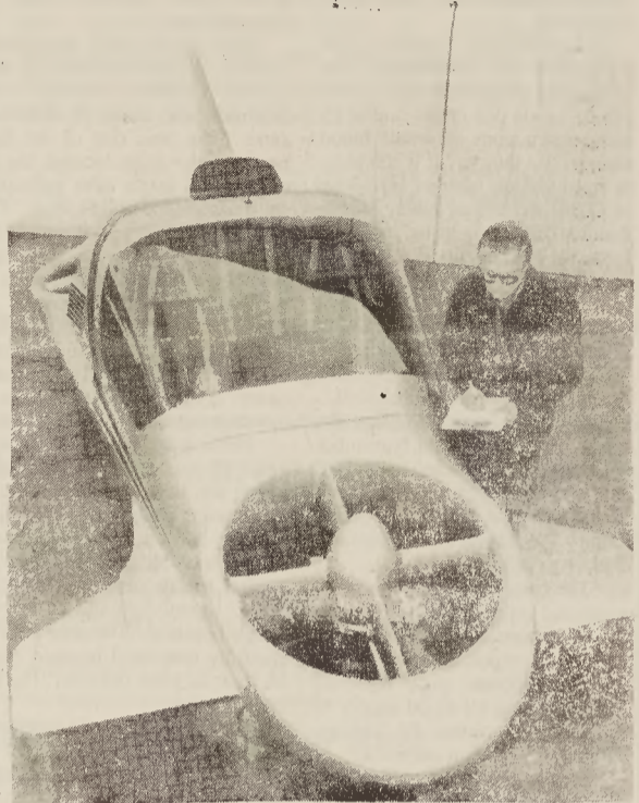
ARLINGTON, WASH. — Fred Barker, president of Flight Innovations Inc. here, checks the front rotors of a prototype Sky Commuter vertical takeoff and landing aircraft. The flying machine is built around an airframe made of super-tough Du Pont Kevlar fiber and graphite. It has a 225-mile range at speeds of about 85 m.p.h. (UPI Photo)
