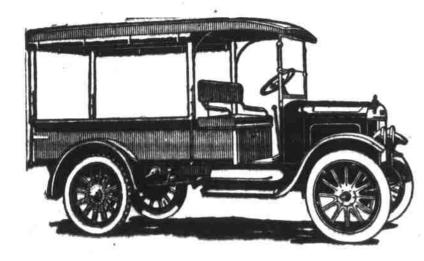
Model No. 9 Express Body, Canopy Top and Curtains Electric Lights, Horn and Generator, Solid or Pneumatic Tires, 1,500 Pounds Capacity \$750.00
