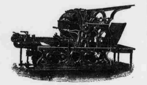
page papers an hour. We do not expect to operate the press that fast, however. The press illustrated below weighs fourteen thousand pounds, the cylinder alone weighing three thousand five hundred pounds. With a larger press we print a larger paper.
