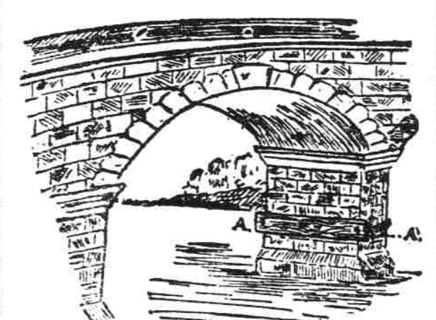
ONE METHOD OF BLOWING UP A BRIDGE.
