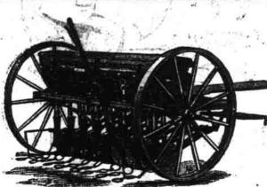
The fertilizer feed in the THE HOOSIER consists of a series of nicely fitted circular plates-one for each disk-arranged to revolve in the hopper at the bottom. The fertilizer is
