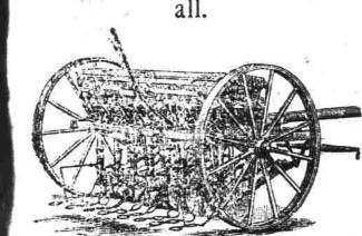
The low hitch on these machines prevents neck weight and causes them to run steadily. The agitator in fertilizer hopper stirs the fertilizer while the machine is in motion and prevents chok-
