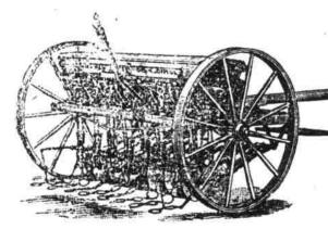
NO changing of cog wheels necessary to increase or necessary to increase or diminish either grain or fertilizer feed. This is done by levers which are in easy reach of the operator.
