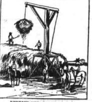
DERRICK FOR STACKING HAY. short end 4 feet, long brace 15 feet,
