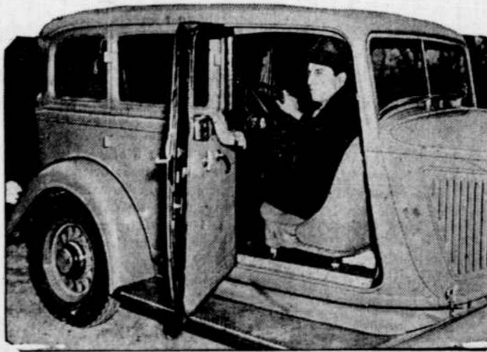
HARRY HARTZ, race driver and automotive engineer, demonstrated an automobile at the Central Park casino, New York, with its body completely reversed, in accordance with his ideas concerning the incorporation of aerodynamic principles into automobile design. His thoroughly revamped automobile, strange as it looks, promises to revolutionize motor car design in that it lowers wind resistance, accelerates speed and saves fuel.
