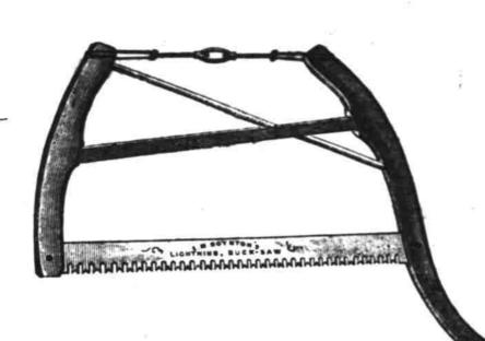
E. M. Boynton's Lightning One man Cross cut. for cutting Wood, Joists, Logs and Timber, and saw-
