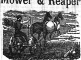
MANUFACTURED BY THE Belvider Manufacturing Co., Belvider, N. J.; has the gearing (or cog wheel) all in an iron case, so as to exclude all grit, dirt, &c. Contains many new and valuable features which do not exist in others. Works well on INCORPORATED, 1850. | CAPITAL \$350,000 smooth or stoney land and is not liable to get out of order.
