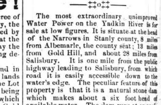
available water. The dam runs at an angle of about 20 or 25 deg. up the river nearly all the way across, gradually diminishing shore. A race of 400 feet in length will add from 12 to 14 additional feet of head, making the grand power of 18 or 20. There is any quantity of building stone and slate of excellent quality, on the premises, easily
