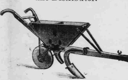
This machine is specially constructed to sow oats by the open to row method. This drill sows outs and guano at the same trip and covers the grain in the bottom of an open furrow. The oats are so protected that they never freeze out or Sprew up. With this machine it is safe to sow oats any time in the fall or winter.
