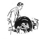
Your tire is carefully mount ed on a tread building mechanism, ready for recapping.
