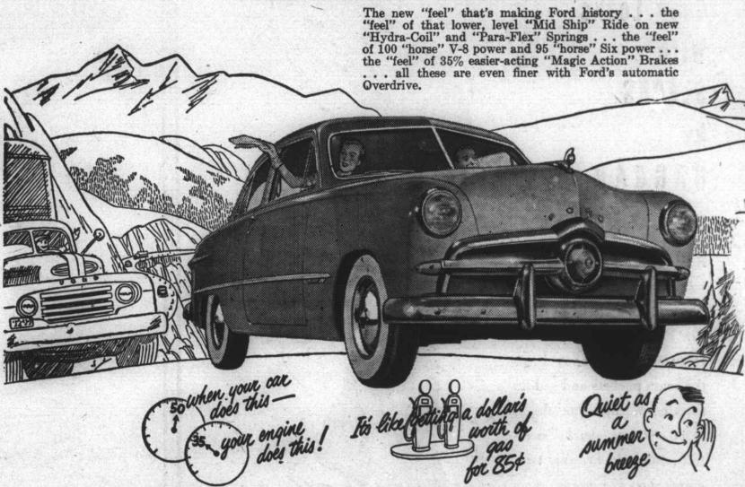
In Overdrive your engine speed drops 80%. Yet your road speed remains unchanged. Your car's doing 50 m.p.h., for example, while your engine's doing only 35.
