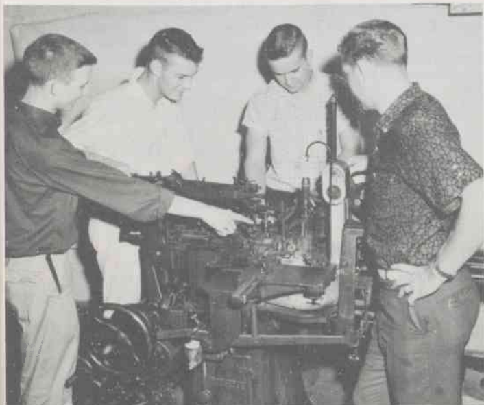
A VALUABLE GIFT — This Monotype has been donated to the Roy Parker School of Printing at Chowan College by Parker Brothers, Inc., of Ahoskie, Windsor, Rich Square, and Gatesville. It has a sales value of $1,500.00 and will save the school a great deal in cost of spacing materials, which this machine makes. It also makes type, which is added saving.
