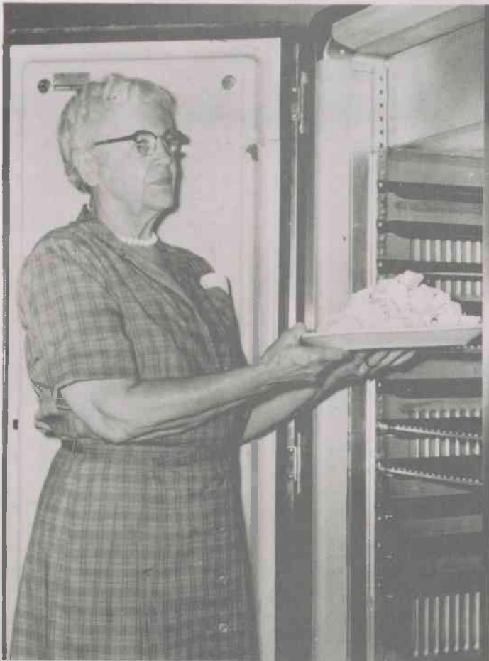
COOLER AND WARMER — Mrs. J. F. Beaman, dietician, is shown at a section of one of the modern cooler-warmers. One half keeps food warm, the other, salads, etc., cool. Food is placed in this equipment in the kitchen and can be taken out at serving sections.
