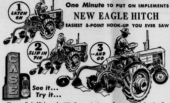
The new Eagle Hitch on the 1950 Case "VAC" tractor takes hold of the new latchon implements and picks them up-fast and easy. Without getting off the seat you just latch on, slip in a pin, and go! You get to the field quicker, finish sooner. Work is done better because the Eagle Hitch keeps implements working at a steady depth in spite of
